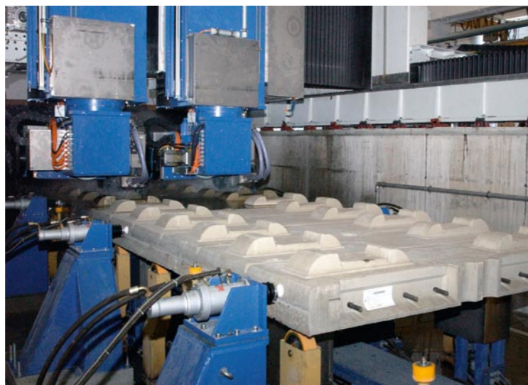
Machining of a roadway element for an ICE railway track: 9 tonnes of concrete precisely clamped.
