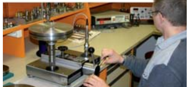
Test technician Robert Rinkart calibrates a pressure sensor by loading it with high-precision weights
