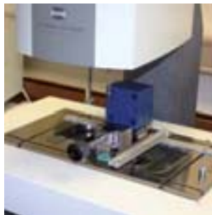
Tactile sensors with ultra-high precision check the size accuracy of a component
