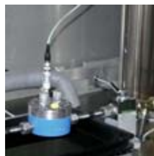
... gear flow meters are tested and calibrated ...
