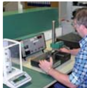
Test technician Bernd Zey executes a surface testing of delivered parts
