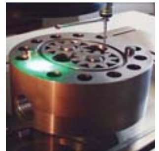
5 µm is the allowed tolerance for these gear wheels
