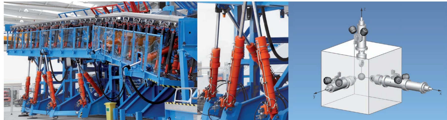
1 | 2 Test stand for wings for airflow simulation 3 | Drawing: Cylinder arrangement in a 3-axis test stand
