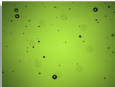
Air bubbles can be seen in images, which are size categorised and removed from particle counts.
