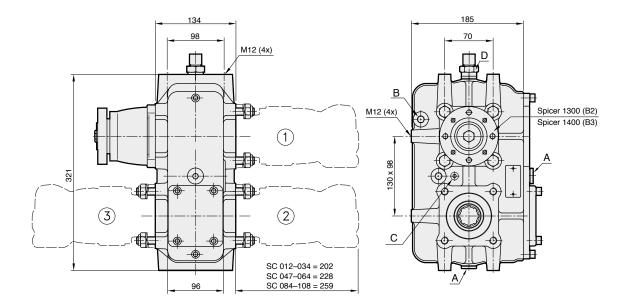
The gearbox must be filled up to the level plug with hypoid oil with intermittent operations.
